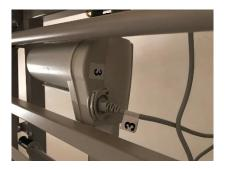
Please be sure to connect the corresponding number to the number on each actuator. Backrest (connected to the control box) = 1, Knee break = 3 and the two Hi-Lo actuators in the head and footboards = 2 & 4. Push the connector fully into the actuator and push in the locking clip until it clicks.
